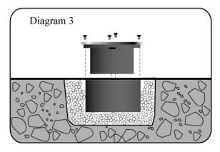
3. After the grout become hard, put the light inside the mounting box and fix them together with 4 pieces of stainless steel bolts.
