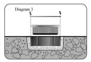
After the grout become hard, put the light inside the mounting box and fix them together with 4 pieces of stainless steel bolt.
